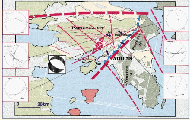
Fig. 2 Model of active tectonic structure of Attica and geodynamic model related to Athens earthquake.
