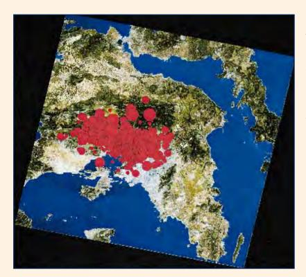
Figure 1. Aftershocks distribution of the well locate aftershocks for the time period Sep. 08 - Oct. 03, 1999, indicating a trending WNW - ESE in consistency with the proposed fault plane solution.
