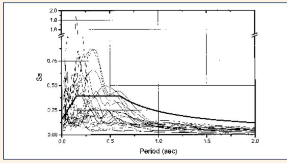
Figure 6. The corresponding spectra, while the dashed line represents the response spectrum adopted by the New Seismic Design Code.
