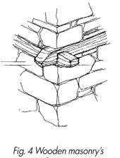
ig. 4 vvooaen masonry s reinforcements.
