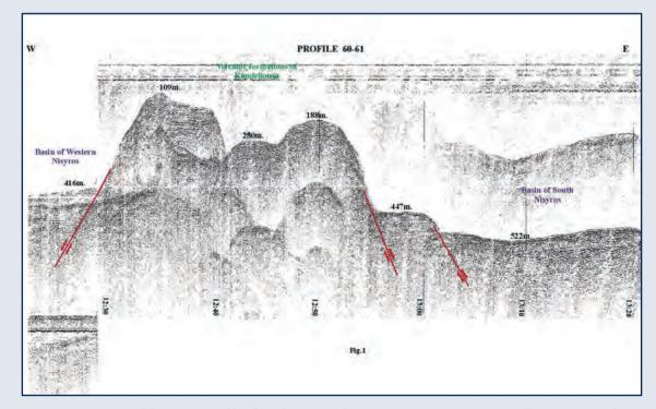
Fig. 1 Representative lithoseismic profile of a submarine volcanic outcrop, using air-gun on R/S "Aegaeo" in the area west of Nisyros Island.
