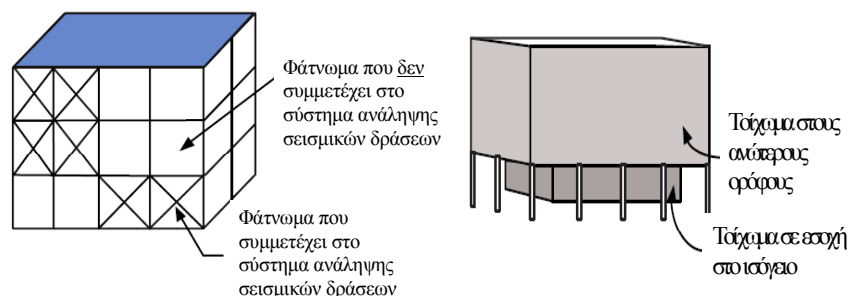
Figure 5.1 Examples of irregularity in elevation: interruption of the structure along its height (setback, left) out-of-plane projection (right)
